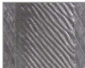
Machined surfaces displaying chatter
