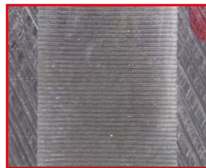
Machined surfaces without chatter
